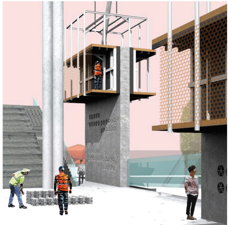
Figure 5. The Imperfect Perforations' concrete 3D printing methodology produces blocks that can be placed in slip-formed concrete shear walls to create ornamental punctures or punctuations.
